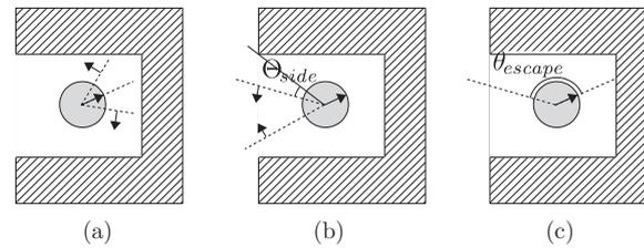
Fig. 5. Finding  $\theta_{escape}$ : (a) search begins from the centre of the front arc and gradually expands in both left and right directions by one resolution each iteration, (b) the aim is to find an angle where all obstacles within  $R_{avoid}$  are beyond  $\Theta_{side}$ , and (c) this angle is set to be  $\theta_{escape}$ .
