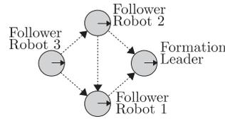
Fig. 1. Inter-robot relationships are represented as a directed graph, where the directed edges go from the follower robots to their local leaders.
