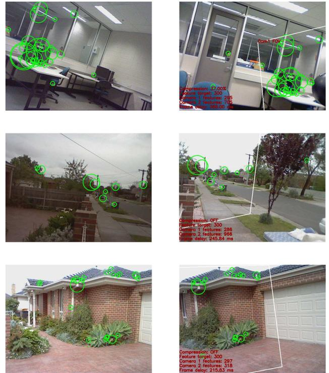
Fig. 4. Screenshot of the tested software. The field of view (FOV) of camera one is plotted as a white outline in camera two. Matching features are shown as green circles. Note that erroneous feature matches, such as those outside camera one's FOV, are detected and disregarded during the homography calculation.
