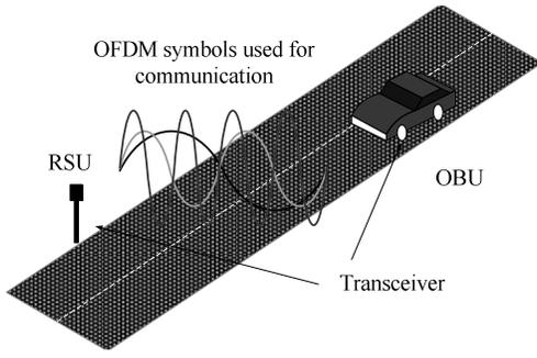
Figure 1. Parts of a WAVE system
