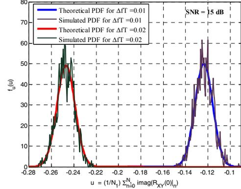
Figure 8. PDF for different  $\Delta fT$  values, when SNR = 15 dB
